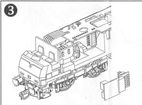
If the PluX12 decoder is used while in digital mode, it is possible to turn on the full beam autonomously. Also the locomotive rear light can be turned off individually or turned on without the front light is turned on. An additional rectangular loudspeaker can be installed in the area of the transformer replica. The loudspeaker is connected to the two soldering pads marked LSA and LSB on the main circuit board.
